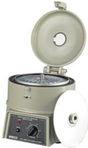
Figure 14.11 Shown here is a centrifuge (left) that spins blood samples that are contained in small glass capillary tubes. The plasma and formed element components (hematocrit) can be seen at in the image above (right).
